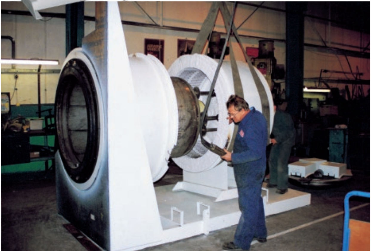
Fig. 24 Assembly of Fibrothal® ROB-segments for a vacuum purge furnace.
