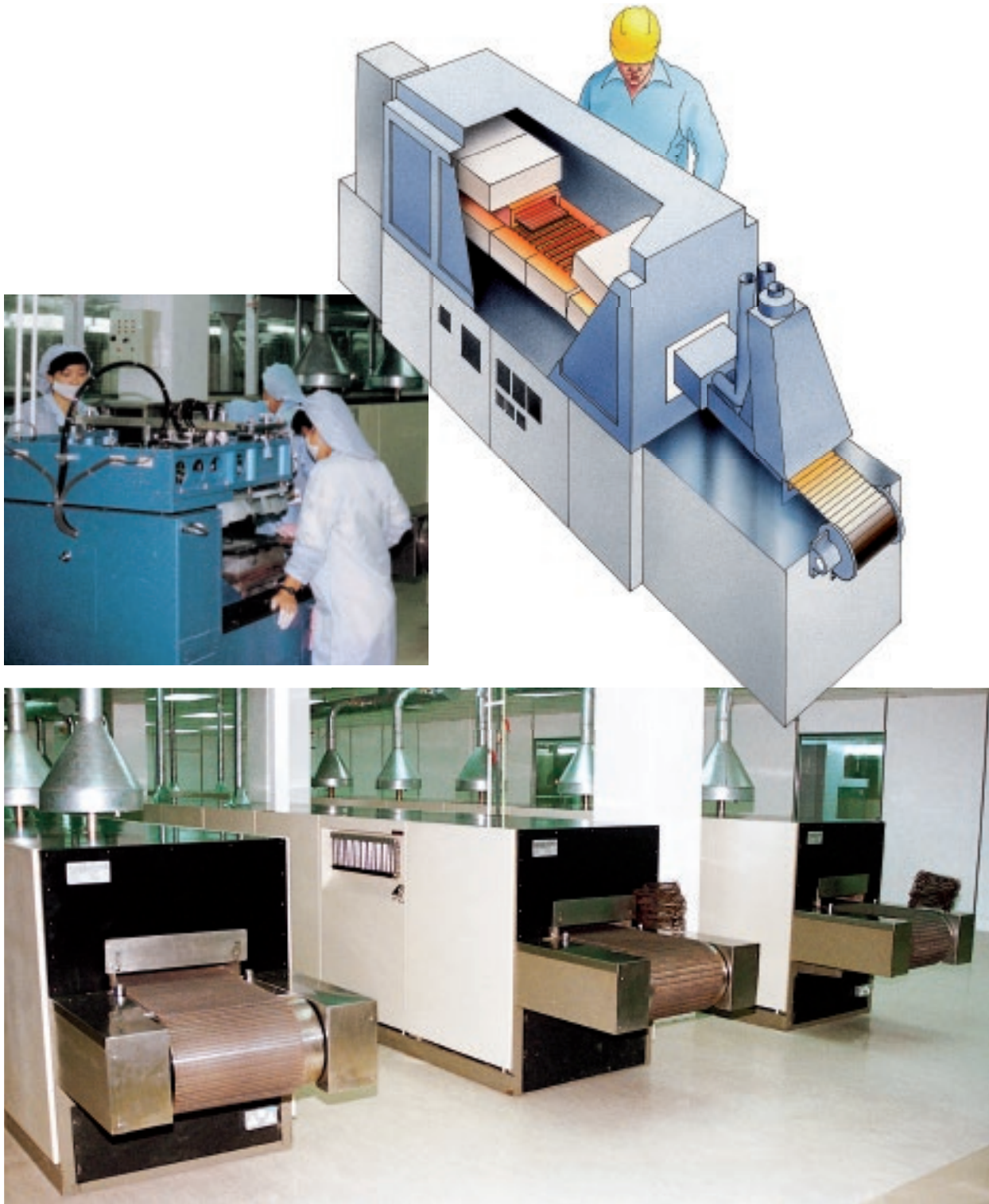
Fig. 25 Fibrothal® modules used in a conveyor belt furnace.
