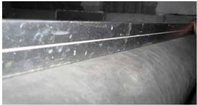
After 1.5 years of service in the hottest zone of a furnace, the W-tube with the burner leg made of Kanthal APMT showed a sagging of 0–2 mm (0–0.1 in).
