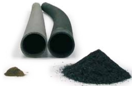
Comparison of tube in Kanthal APMT vs. tube in Fe-35Ni-25Cr after 2300 hours at 1100°C (2010°F). The FeNiCr tube is severely contaminated with oxide flakes.
