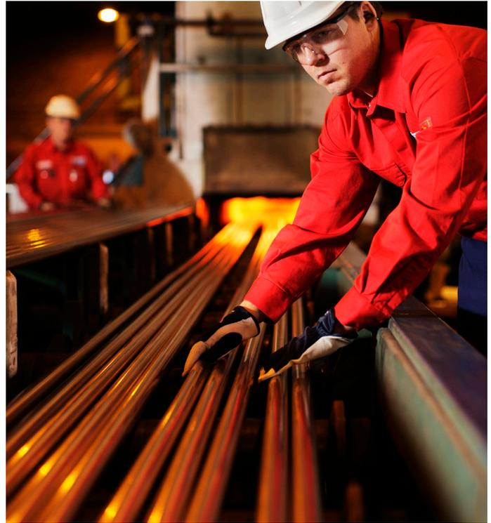
*Furnace rollers made from Kanthal APMT in a Swedish tube mill installation proved to have a service life of up to four times longer than conventional furnace rollers.*
