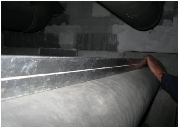
After 1.5 years of service in the hottest zone of a furnace, the W-tube with the burner leg made of Kanthal APMT™ showed a sagging of 0–2 mm (0–0.1 in).
