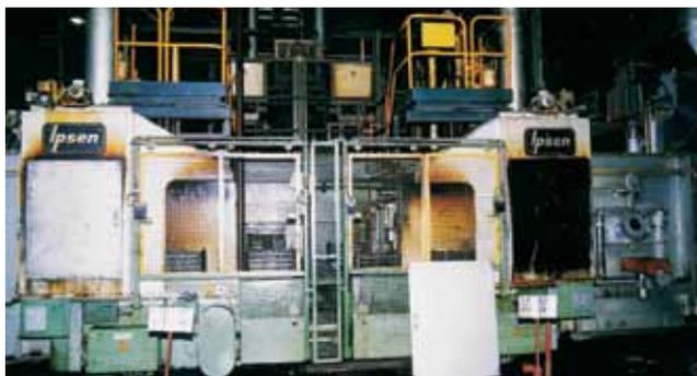
*One of the four gas heated continuous furnaces at Gearbox. Kanthal APM tubes are installed as inner and outer tubes.*
