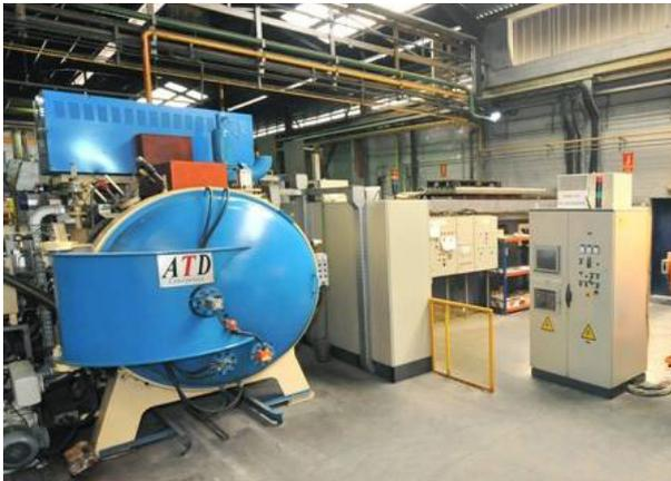
The 240 kW continuous hardening line at Badia S.A. in Barcelona heated by 48 Kanthal® Super electric heating elements.
