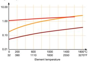
Electrical resistivity compared to element temperature for Kanthal Super ER, Kanthal Super 1800 and molybdenum shows the high room temperature resistivity.
