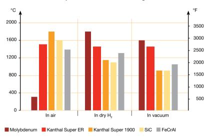
The data should be considered as approximate, since maximum furnace temperature depends on surface loading, gas-velocity, dew point, vacuum level and etc.
