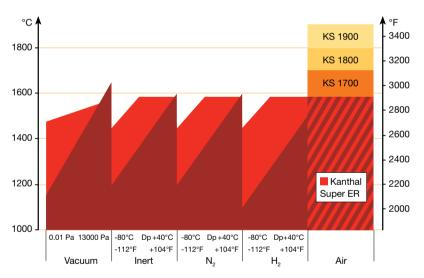
The diagram is a guide to maximum temperatures in different atmospheres depending on dew point, vacuum and etc.
