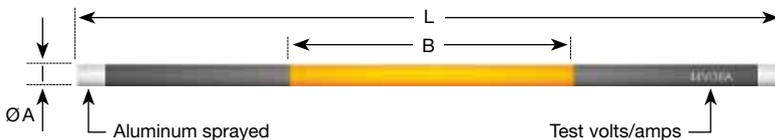
Fig. 1 Standard dimensions for Kanthal Globar SD elements.
