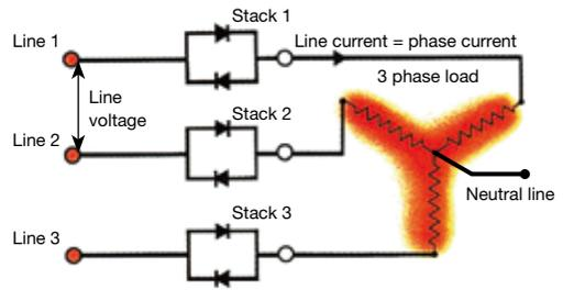
**Three-phase, four-wire, star-connection (phase-angle firing)**
