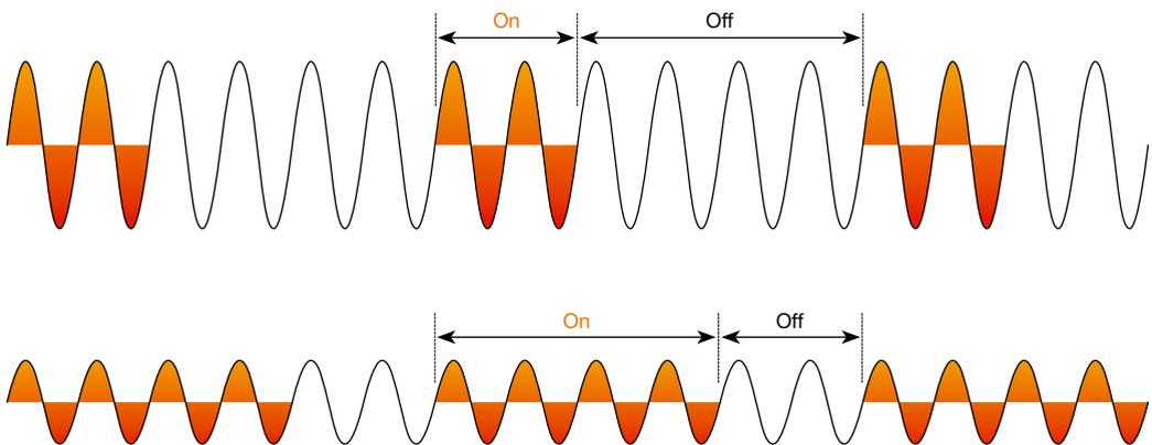
Fig. 18 Fast-cycle firing.
