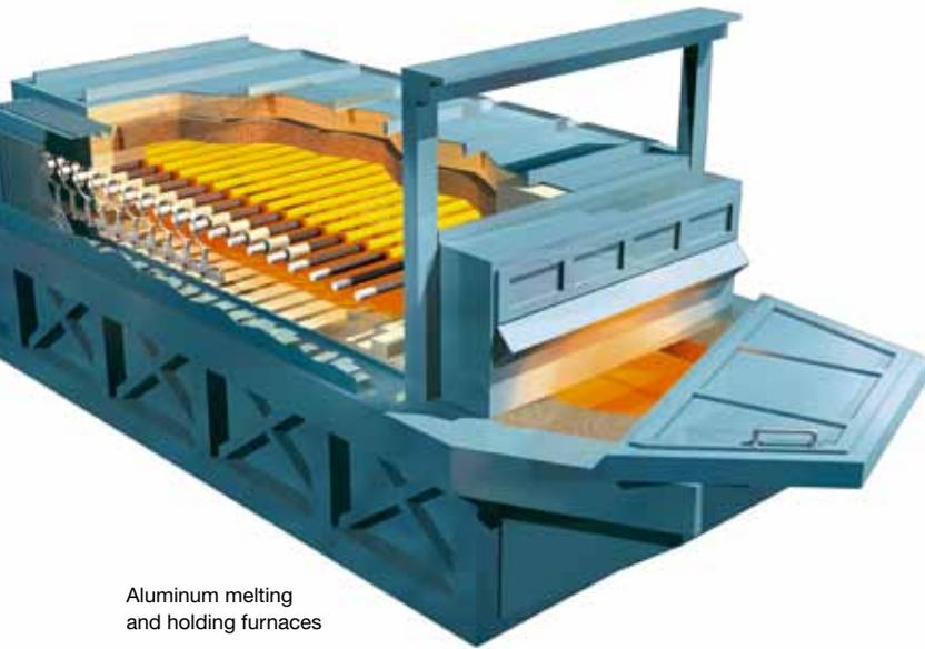
Aluminum melting and holding furnaces
