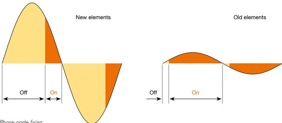
Fig. 13 Phase-angle firing.
