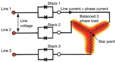
**Three-phase, three-wire, star-connection (phase-angle firing)**
