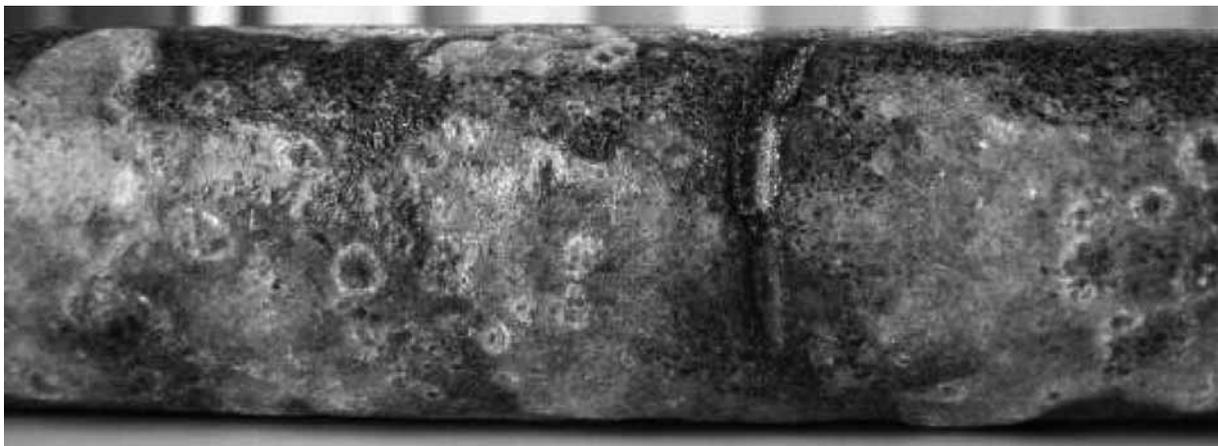
Conventional SiC element with eroded element surface.
