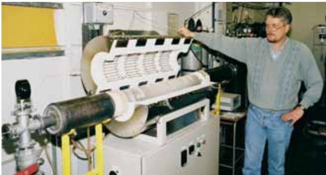
*The new tube furnace at KIMAB consists of six Superthal half-shells mounted into two hinged cassettes. The metallic tube in Kanthal APM has an outer/inner diameter of 128/117 mm (5/4.6 in).*
