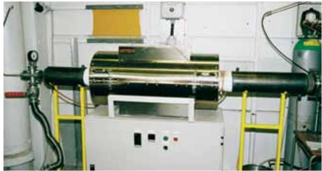
*The furnace is equipped with a multi-gas feed system that includes vacuum and various protective gases. The tube is water-cooled outside the heating chamber.*
