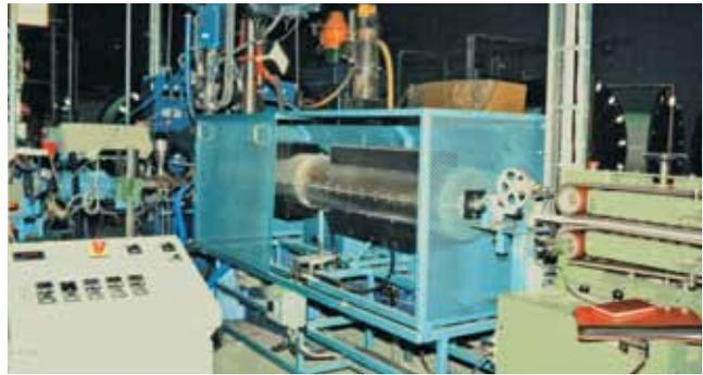
*Uponor evalPEX pipes are heated in two Superthal cassettes before the diffusion barrier is applied.*
