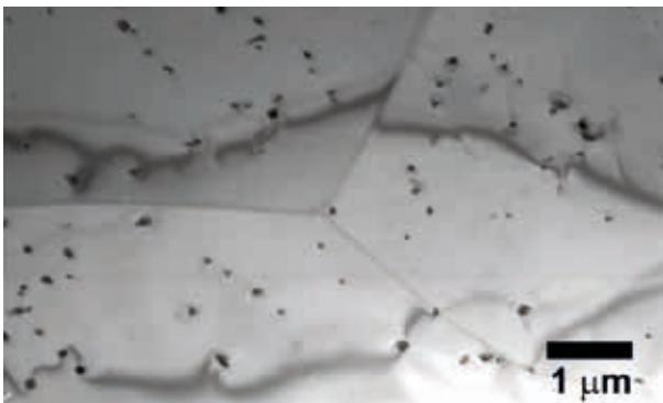
The unique dispersion of small refractory inclusions in Kanthal® APMT improves creep properties.
