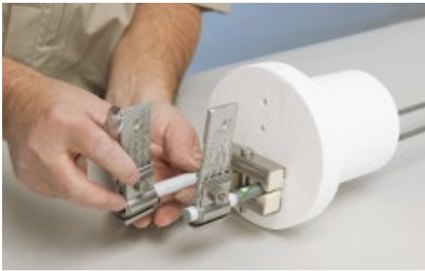
4. After packing heavy-duty ceramic fiber loosely into the recesses of the terminal holes...
