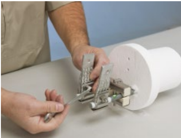
6. When determining the position of the element holder, it is of the utmost importance to ensure that the tapered transition between terminal and heating zone comes fully below the hot face of the furnace lining. If not, there is a risk that the part of the heating zone which is inside the lining may become overheated. When connecting the installed elements, the aluminum braids should first be bolted to the elements and then to the busbars.
