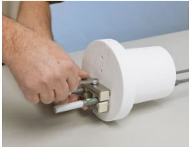
5. ...single- or two-shank element holders should be fixed to the terminals.
